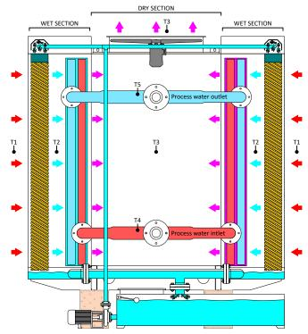
FLOW DIAGRAMS For proper methedology of process cooling, below ginve are few diagrams on selections of right equipment.
